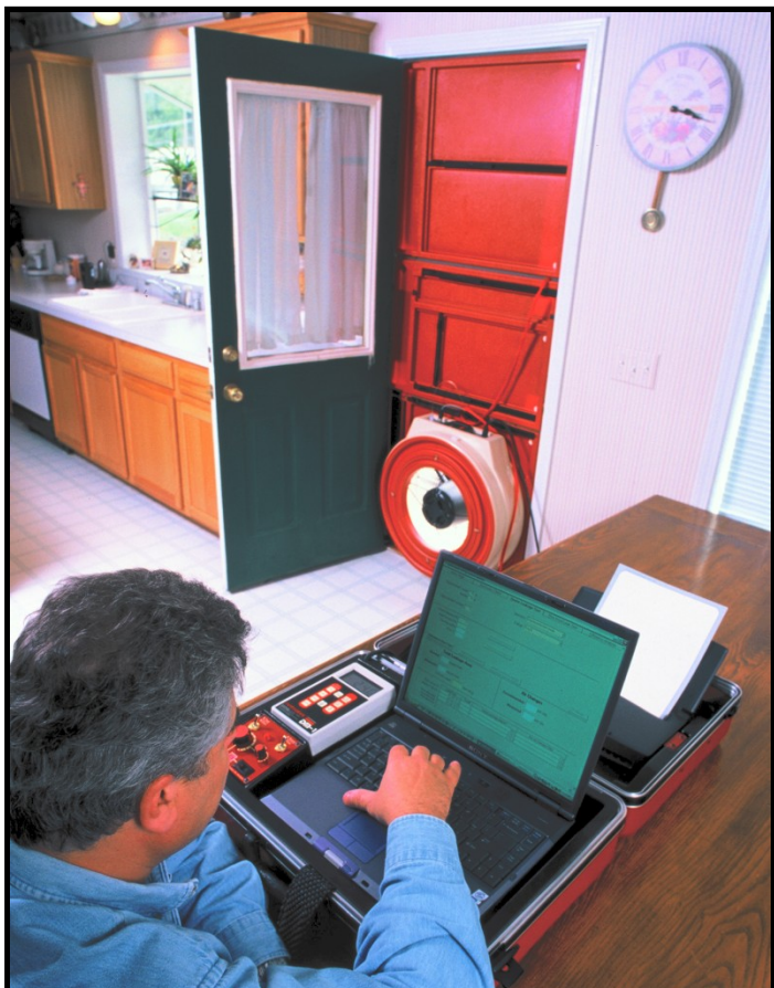
The Infiltrameter test pinpoints air leaks in your house and duct system
